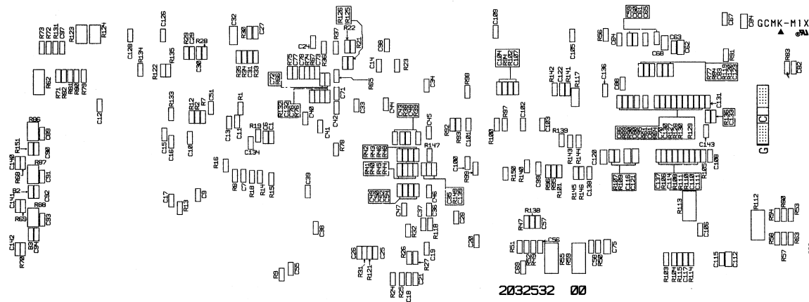
Figure 7-3. Component Layout - C304MAIN
